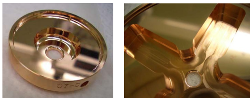
Figure 6: Typical disk-shape cells. Left: undamped cell and right: heavily damped cell with magnetic coupling.
