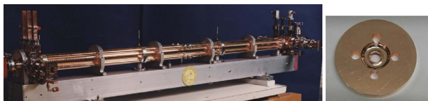
Figure 3: 1.8m RDDS1 structure and constituent cell.
